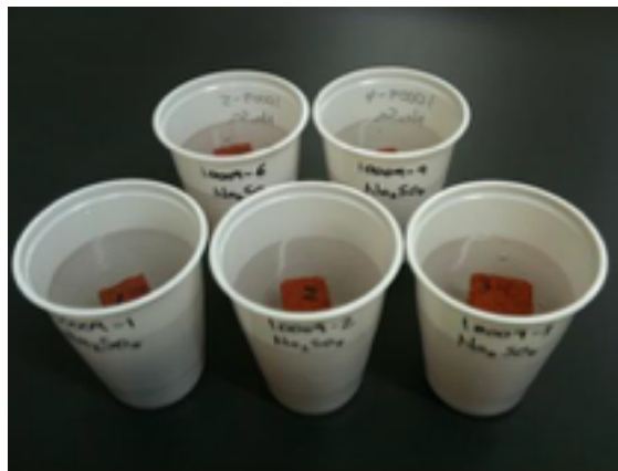
Samples soaking in salt solution
