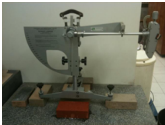
The TRRL rubber slider ready for release over wet paver
