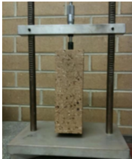
Measuring frame with micrometer
