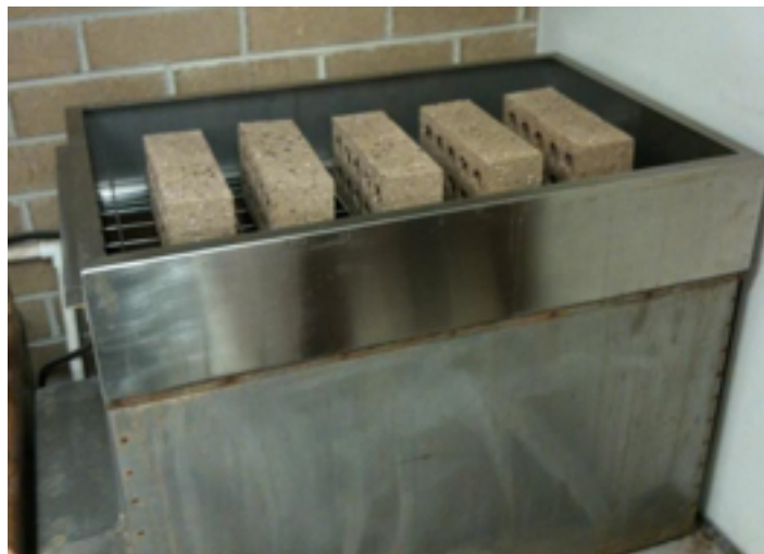
Bricks loaded ready to be steamed
