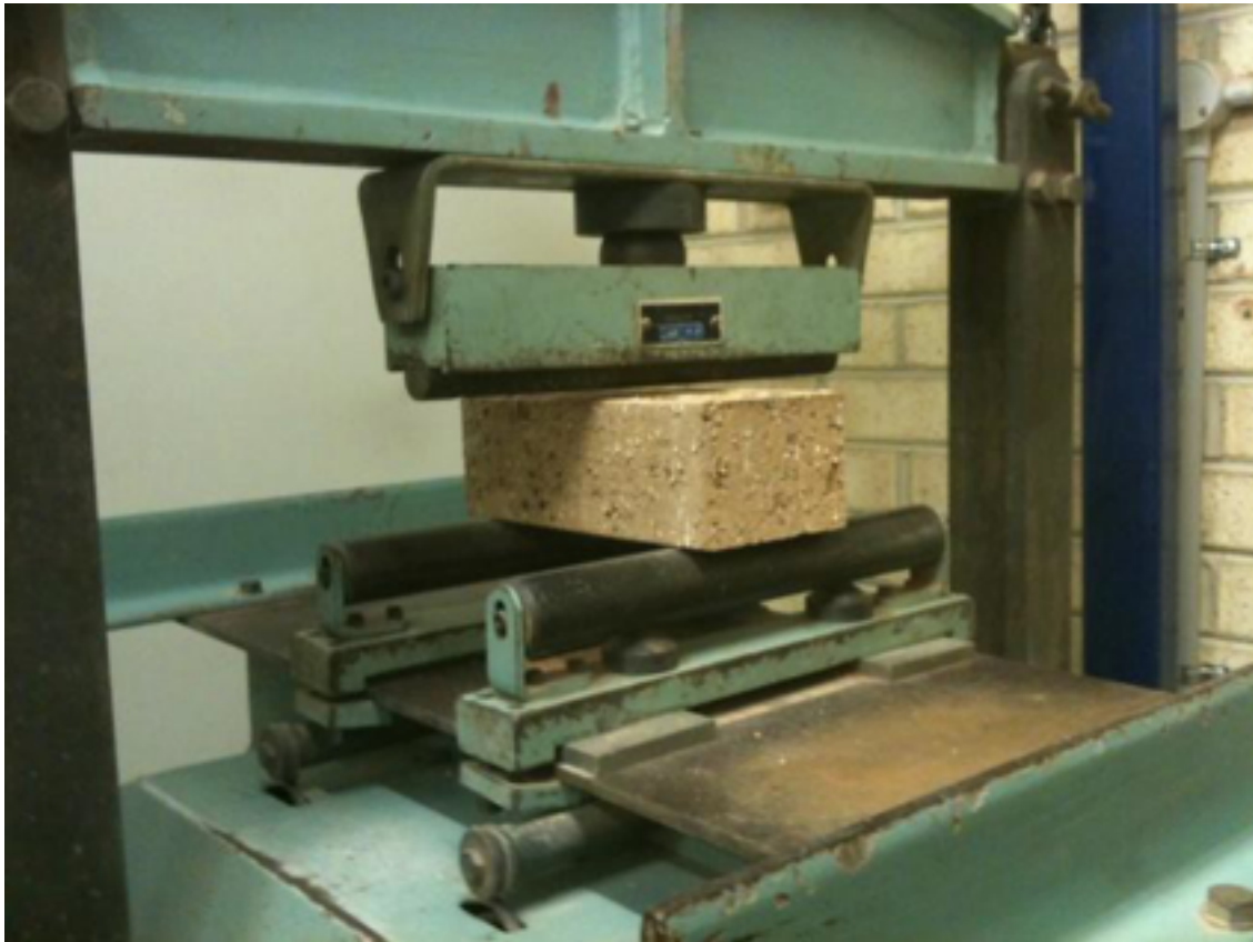
Sample is broken in half by a hydraulic bar
