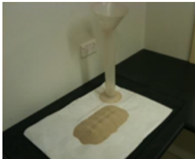
The brick is removed and the sand collected
