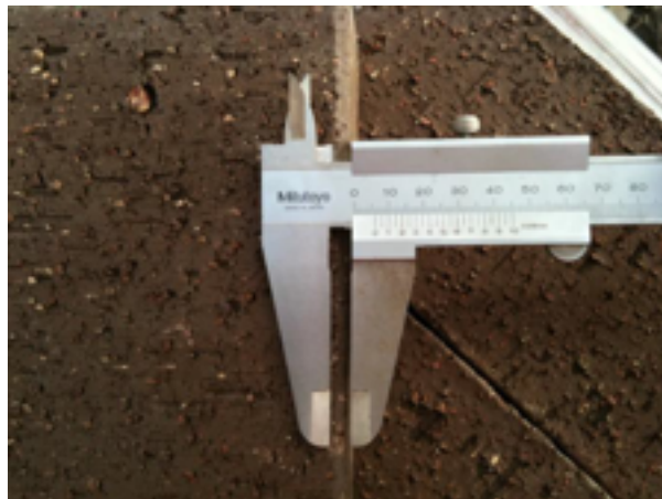
5.9mm chip in edge is acceptable
