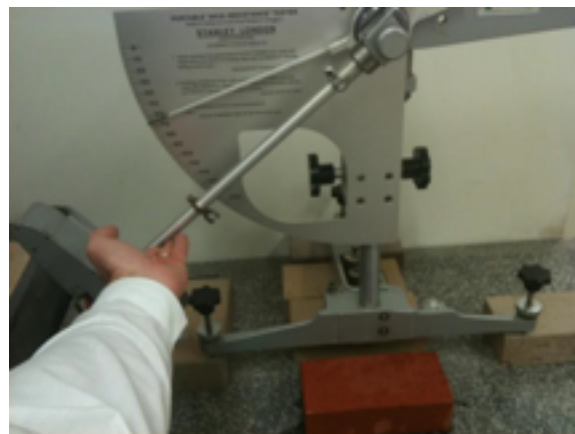
British Pendulum Number (BPN) result is read directly from the scale on the machine
