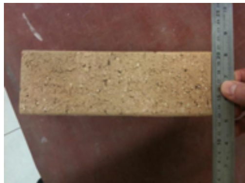
Distortion on Perpend
