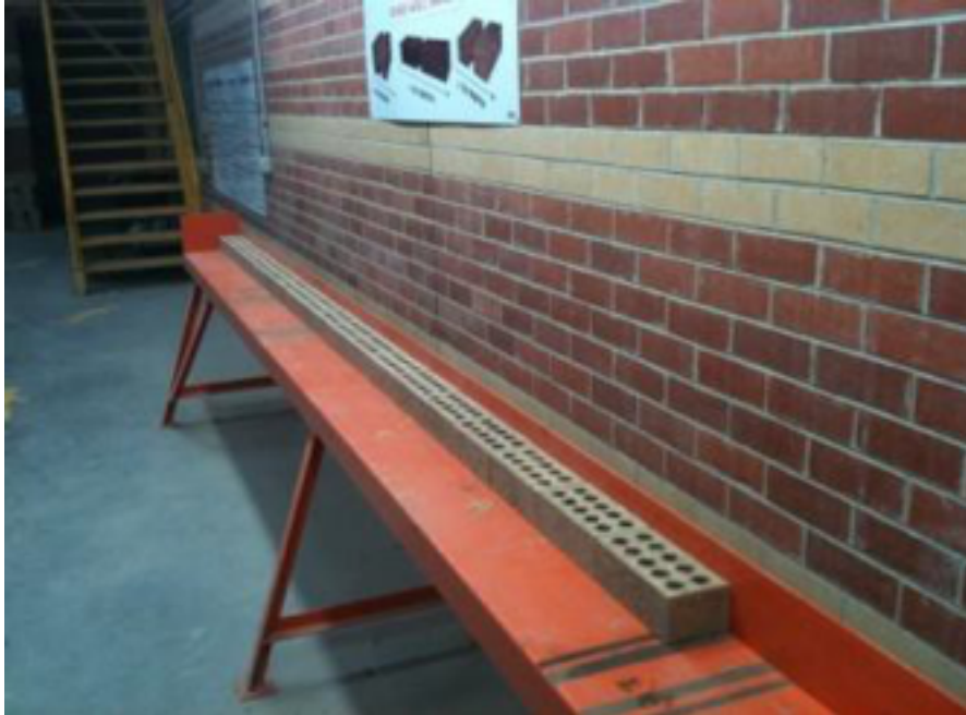
Length is tested over 20 bricks placed end to end – Standard equals 4,600mm \pm 60mm
