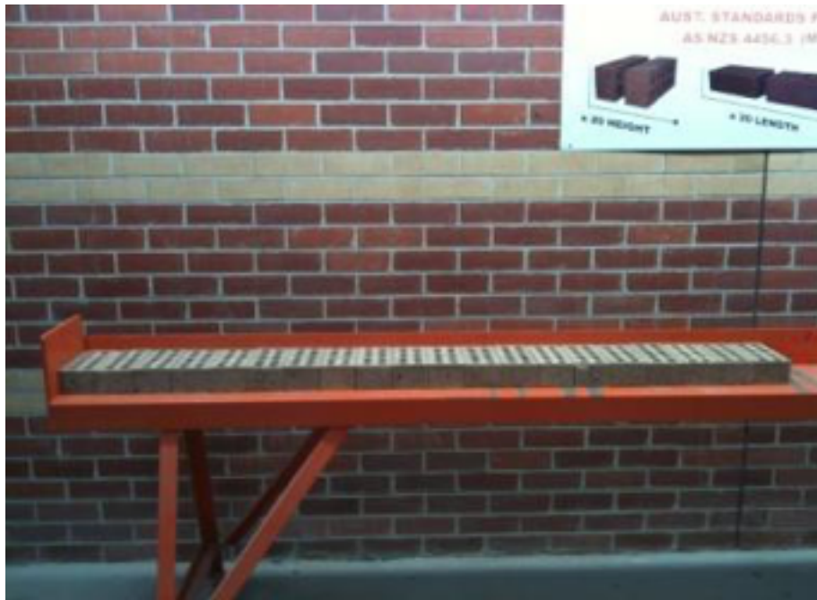
Width is tested over 20 bricks placed side by side 2,200mm \pm 40mm
