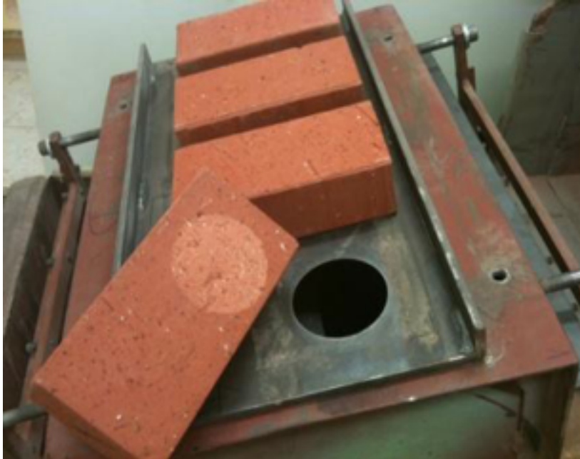
The pavers showing the simulated wear after 3600 revolutions
