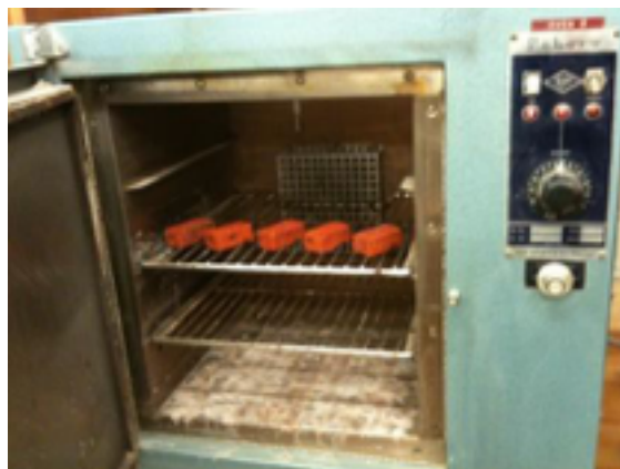
Samples drying to crystallise salts
