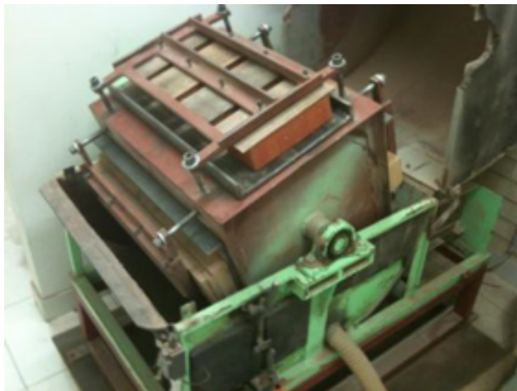
The pavers are clamped to the tumbler ready to rotate (4 pavers on each side of the drum)
