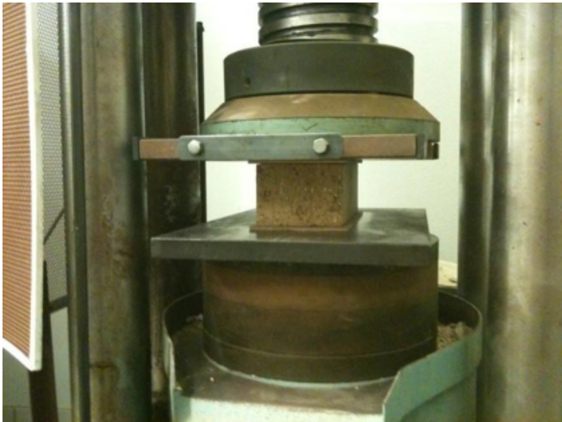
The brick sample is crushed in a hydraulic press
