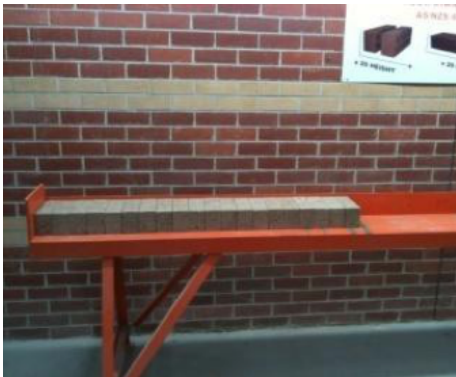
Height (thickness) is tested over 20 bricks placed top to bottom 1,520mm \pm 40mm
