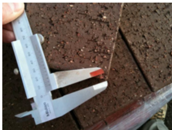
9.4mm chip in corner is acceptable
