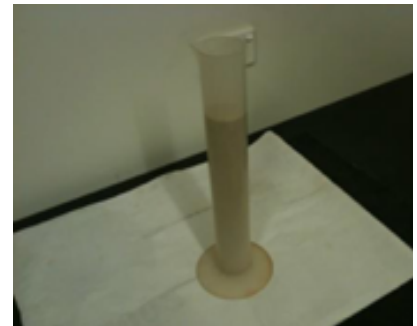
The sand volume is measured
